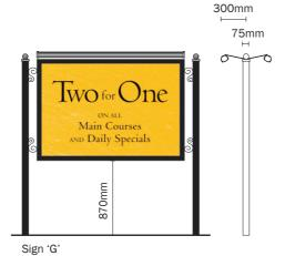
Description - Double sided twin post sign Materials - Aluminium, Illumination - Externally illuminated LED pelmet lights. Panel size - 1,760mm x 1,210mm Cap height for 'T' of TWO= 250mm
