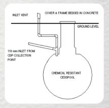
If a manufactured cesspool is chosen, it should be installed by a competent builder in accordance with the manufacturer's instructions (incorrectly installed cesspools may either split or float out of the ground). A suitable hatch and cover must be provided to allow emptying of the cesspool. The cover should preferably
