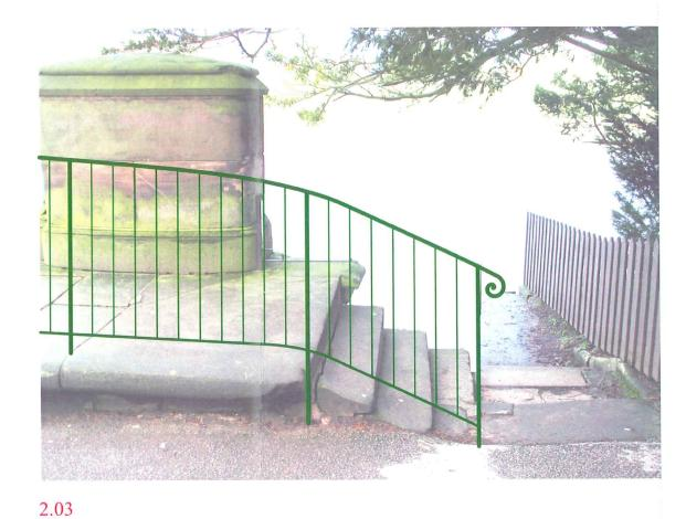
Type 1 Fence with handrail set 900mm above nosings and with transition to 1100mm high fencing at top
