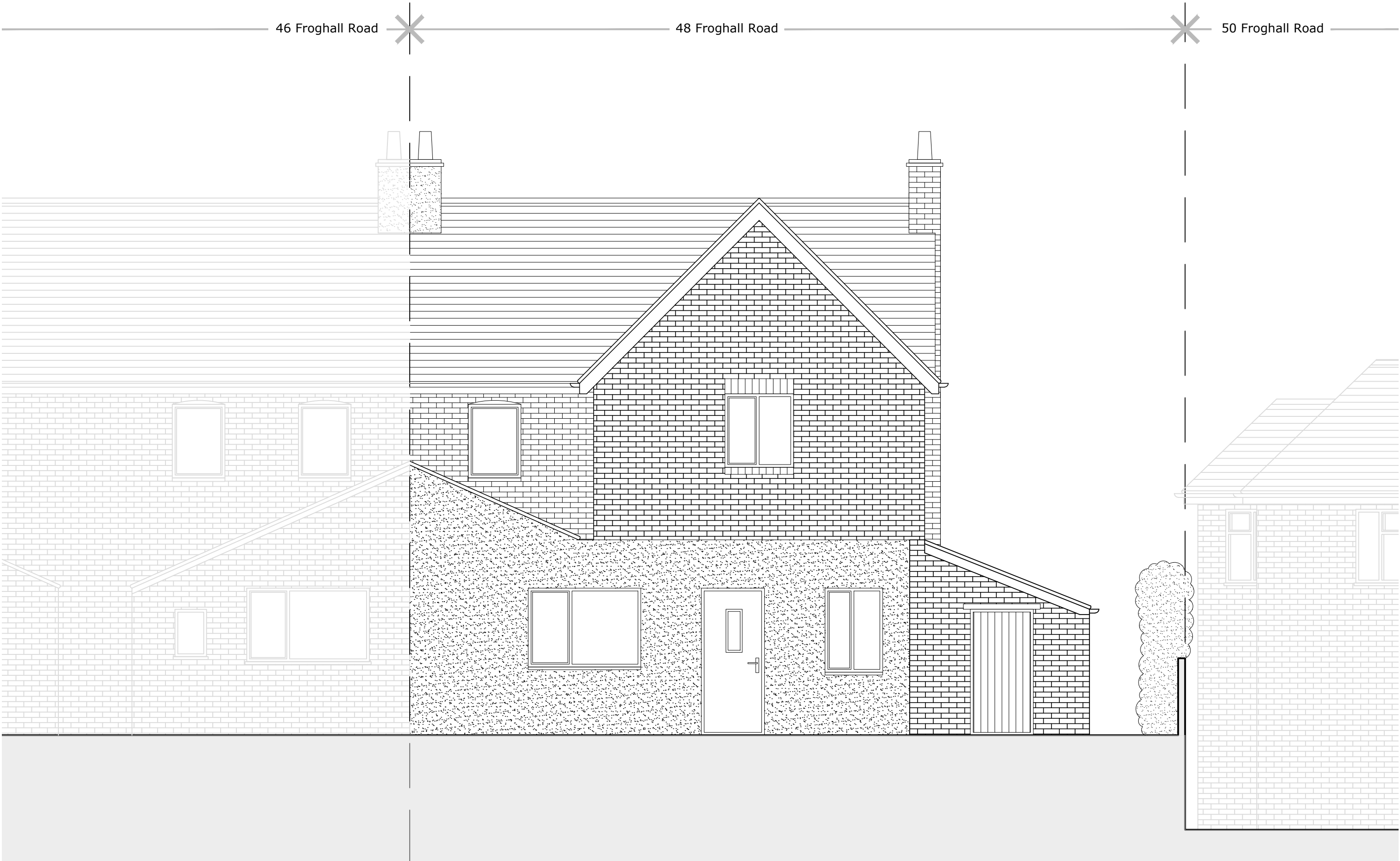
rear elevation (east facing) as proposed 1:50
