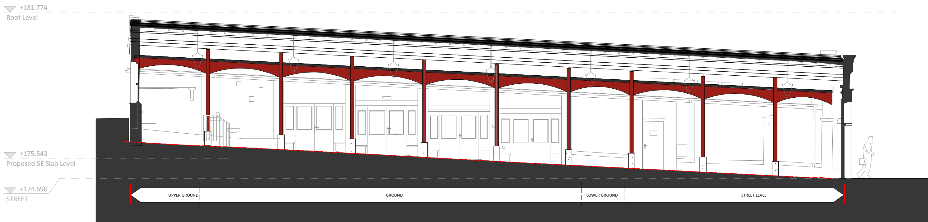
Planning Section B-B - Existing Long Section 1 : 100
