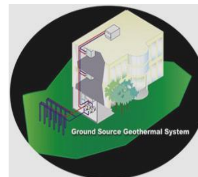
Ground Source Heat Pump Installation
