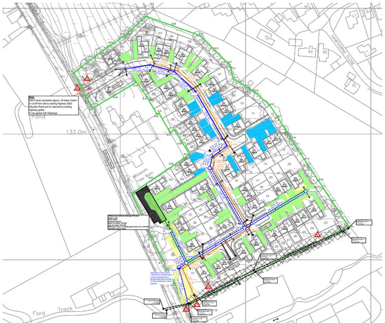
Figure 2- current drainage layout plan (drawing C1941 C-SK03 rev. J)
