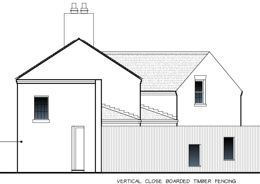
EXISTING SIDE (N) ELEVATION 1:100
