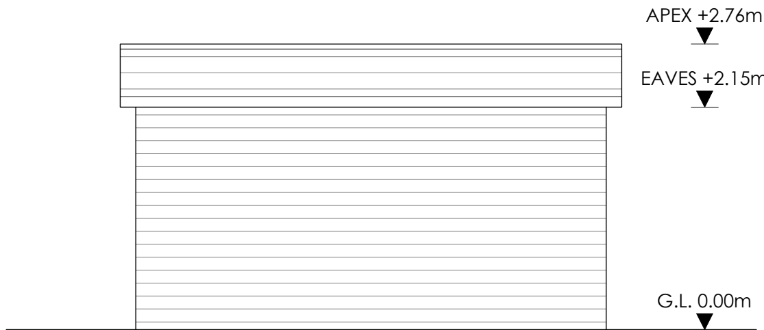
REAR ELEVATION (SCALE 1:50)
