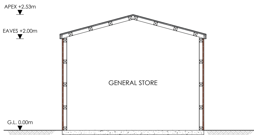
TYPICAL SECTION (SCALE 1:50)
