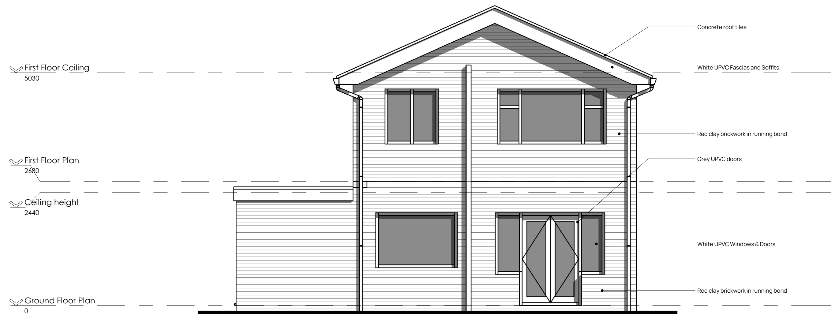
Elevation 3 - Rear Elevation 1 : 50
