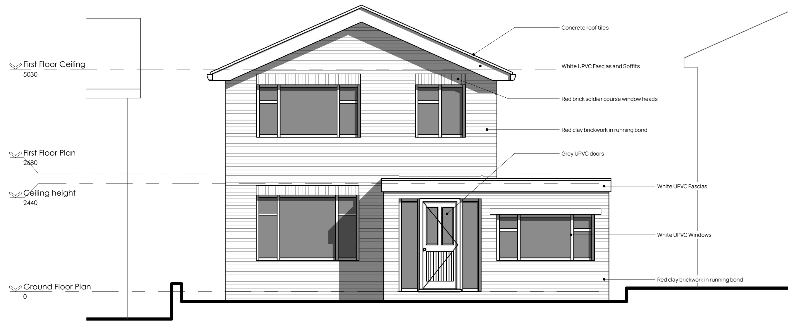
Elevation 1 - Front Elevation 1 : 50
