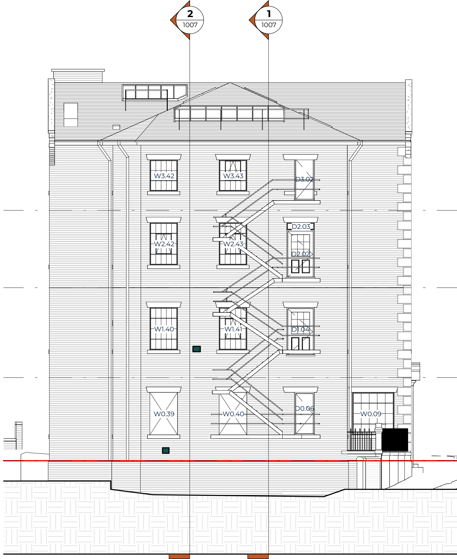
Existing Side Elevation (E) 1:100
