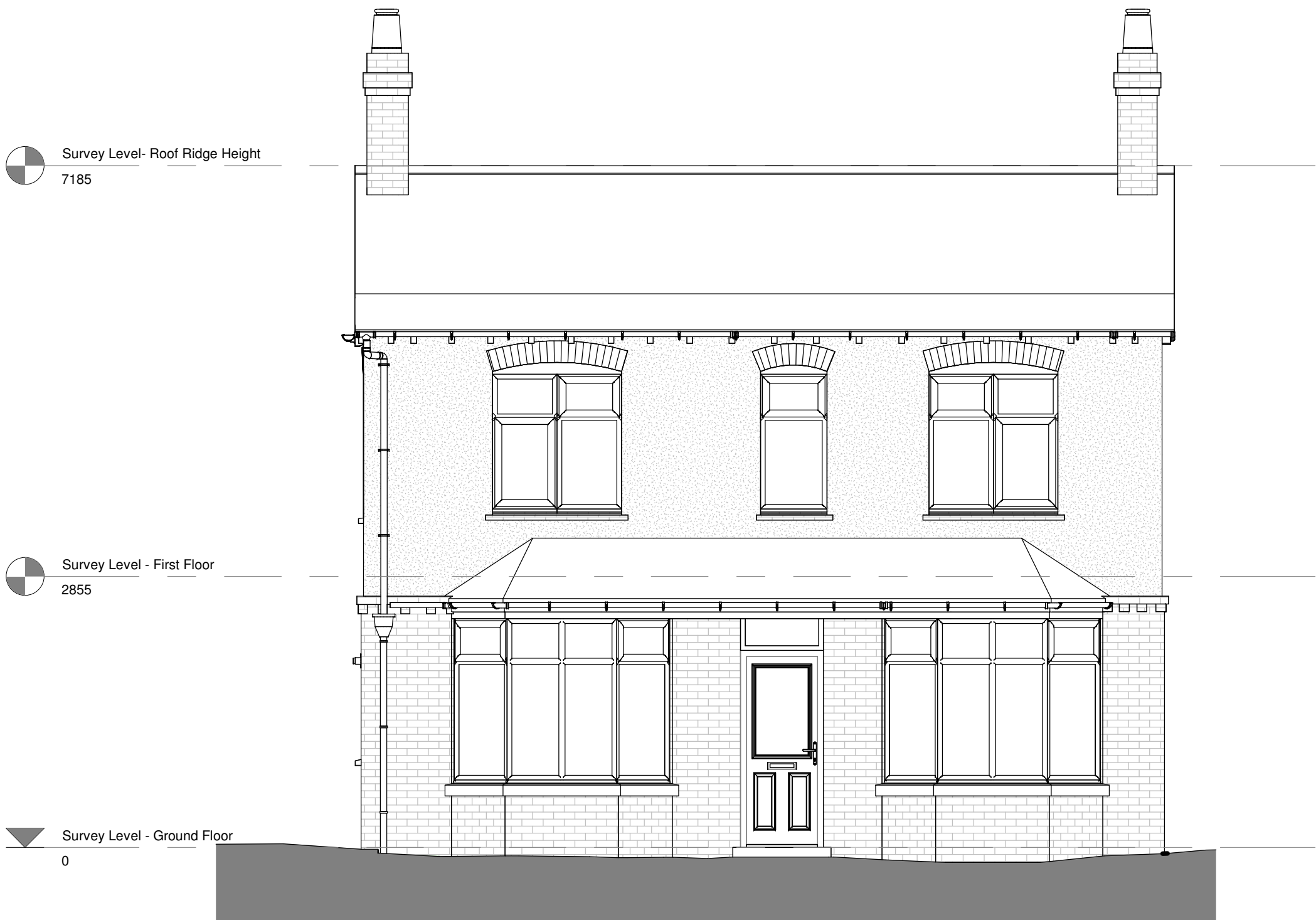
Existing Front Elevation (North East Facing) 1 : 50
