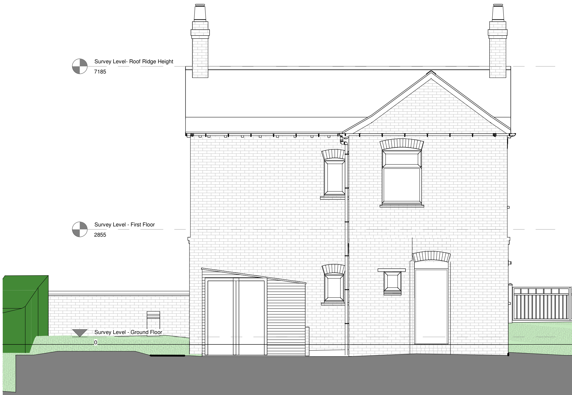
Existing Rear Elevation (South West Facing) 1 : 50
