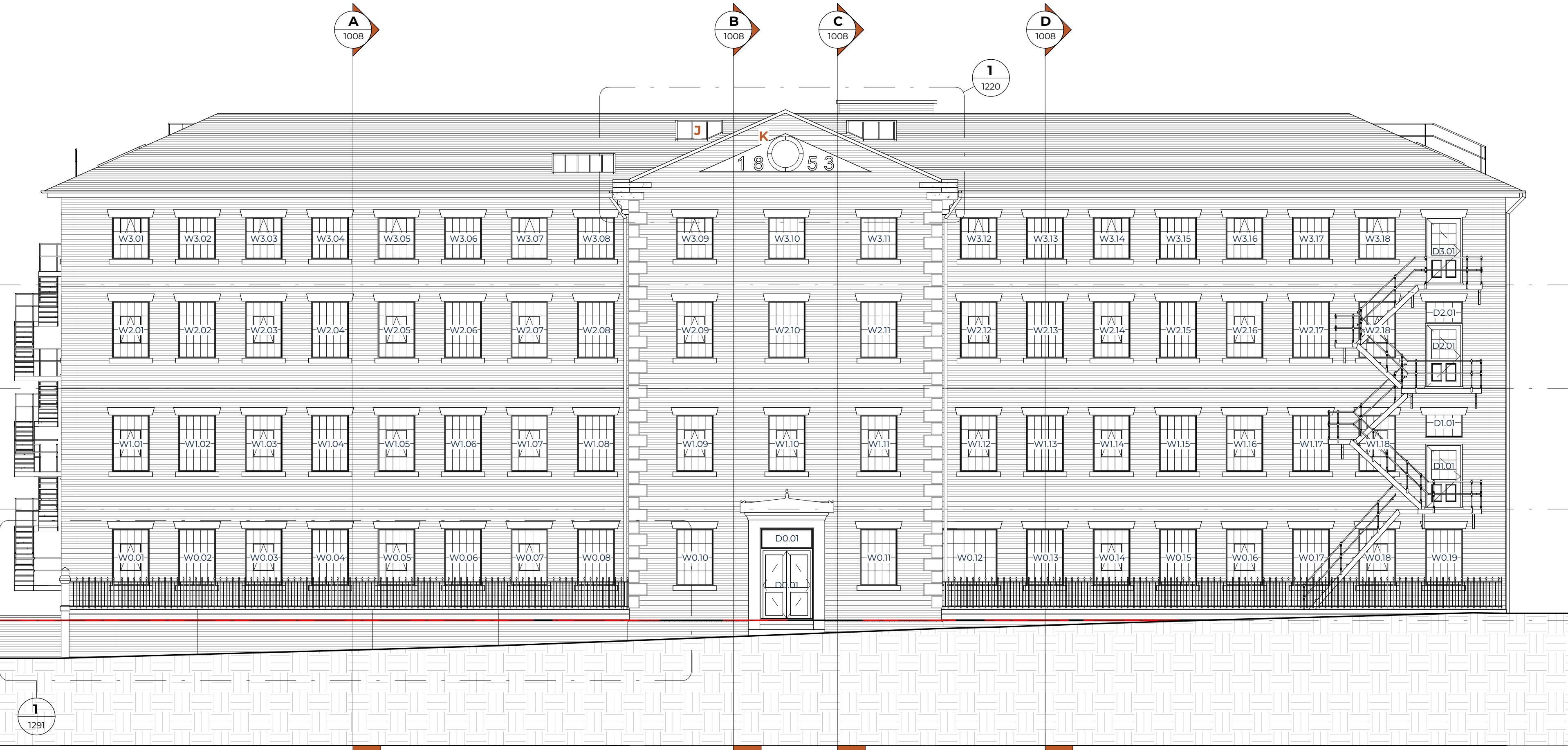
Existing Principal Elevation (S) 1:100
