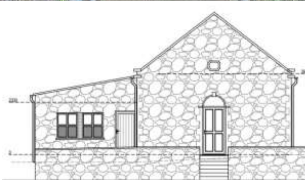
Existing North Elevation
