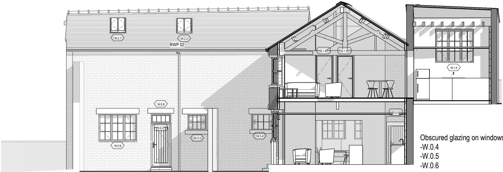
East Elevation onto Central Courtyard as proposed
