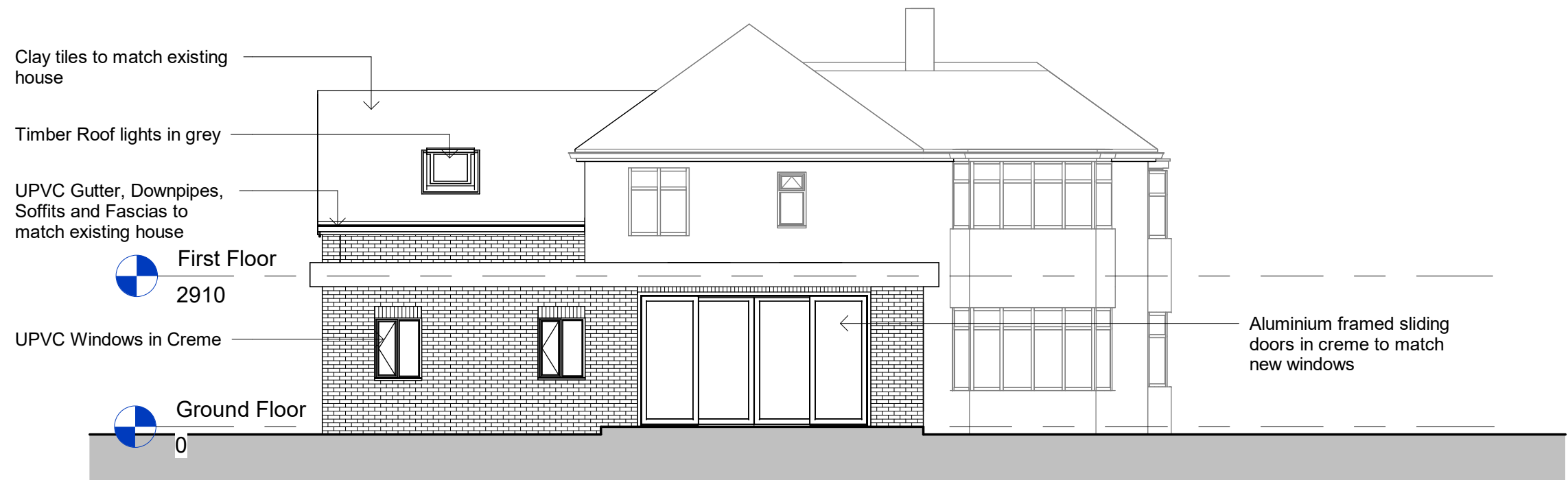
1 North Elevation as Proposed SCALE 1 : 100
