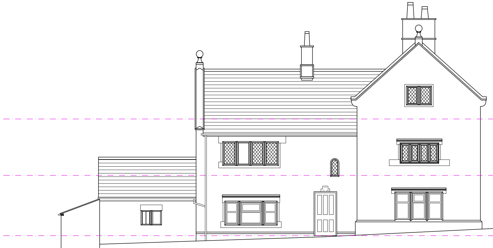
Rear Elevation as Existing 1:100
