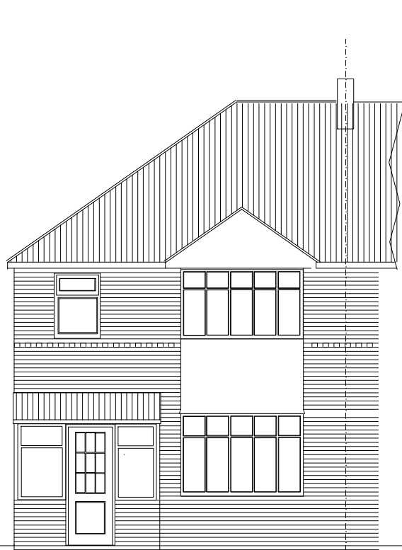
Existing Front Elevation
