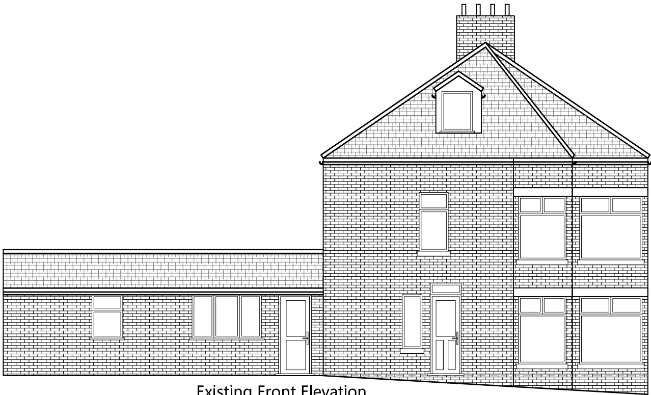
Existing Front Elevation Cruso Street
