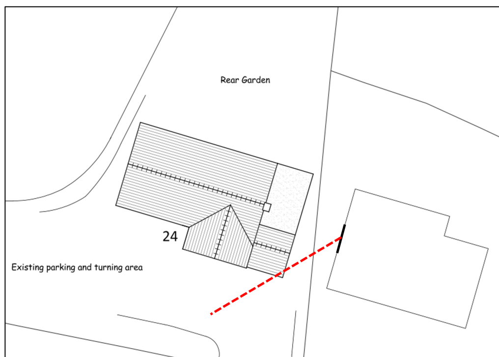
Figure 2 – Application of SMDC 45 degree standard
