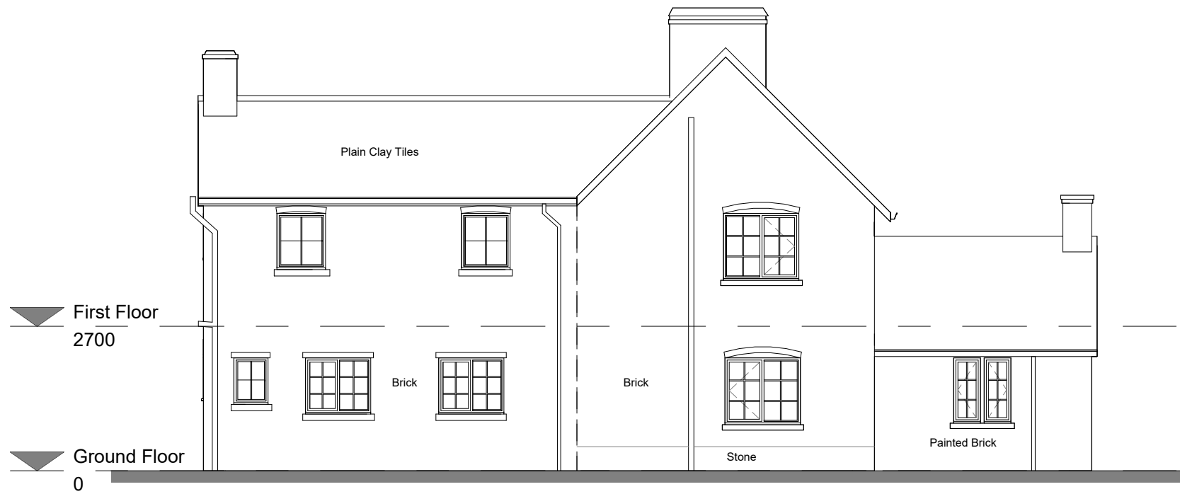
Existing Rear Elevation 1 : 100
