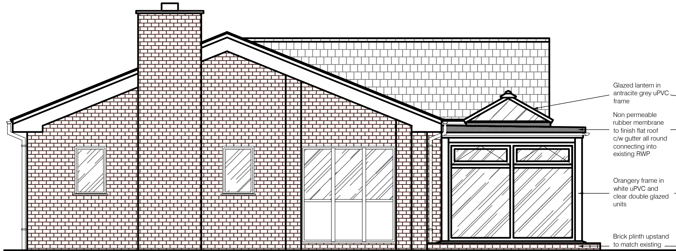
1 SOUTH-WEST FACING ELEVATION
