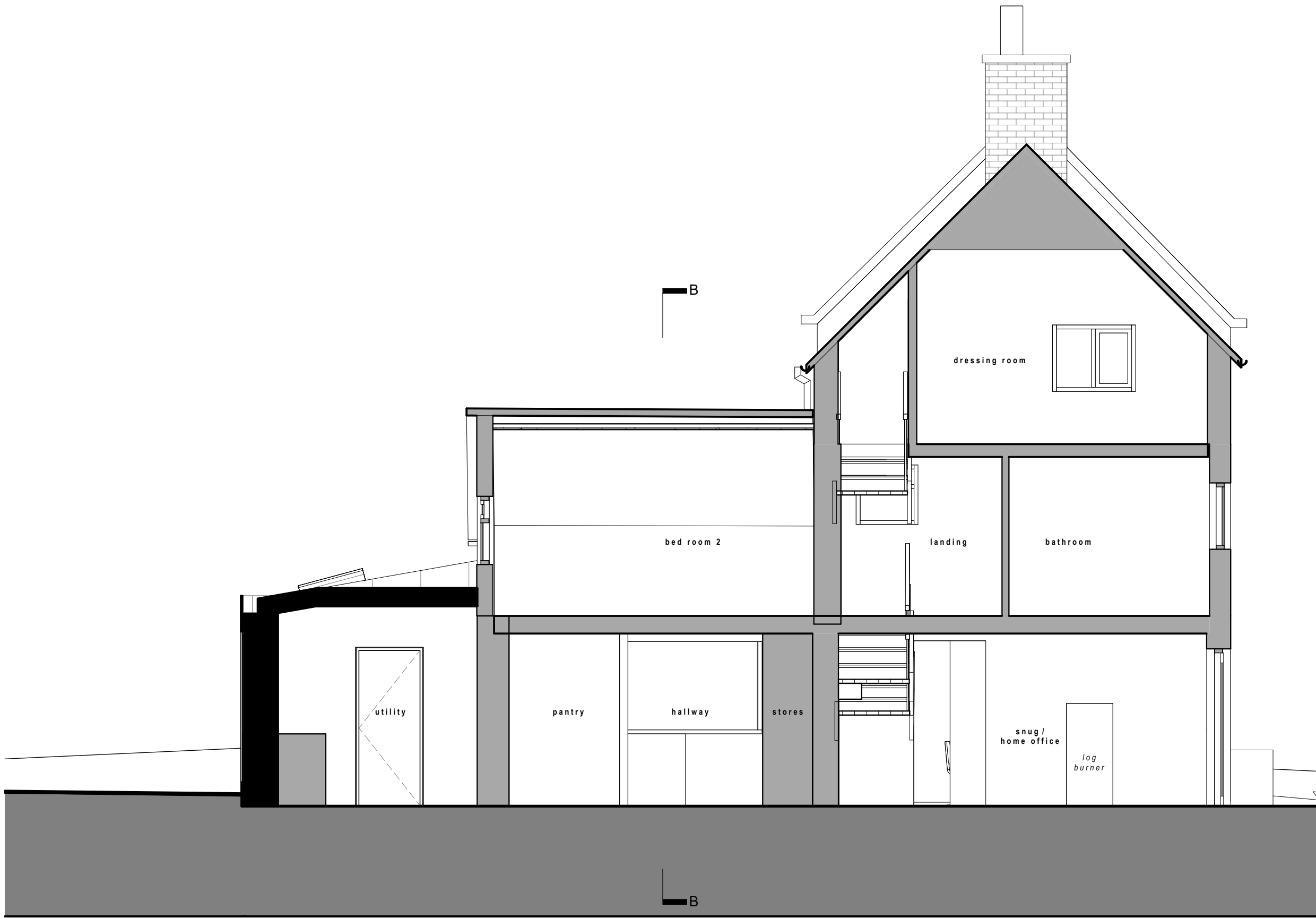
section A-A 'as proposed'
