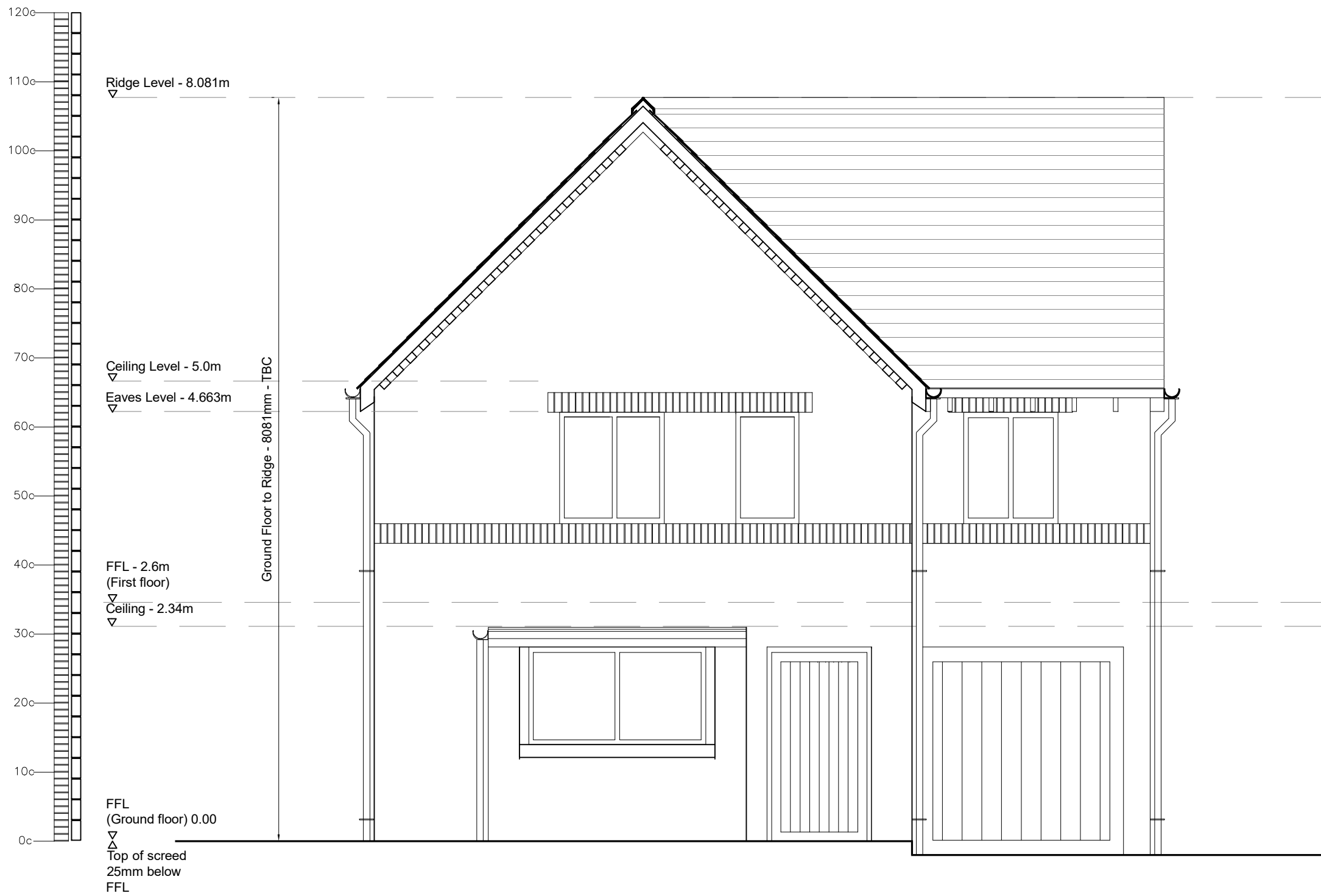
Existing South-West Standalone Elevation 1 : 50 @ A1
