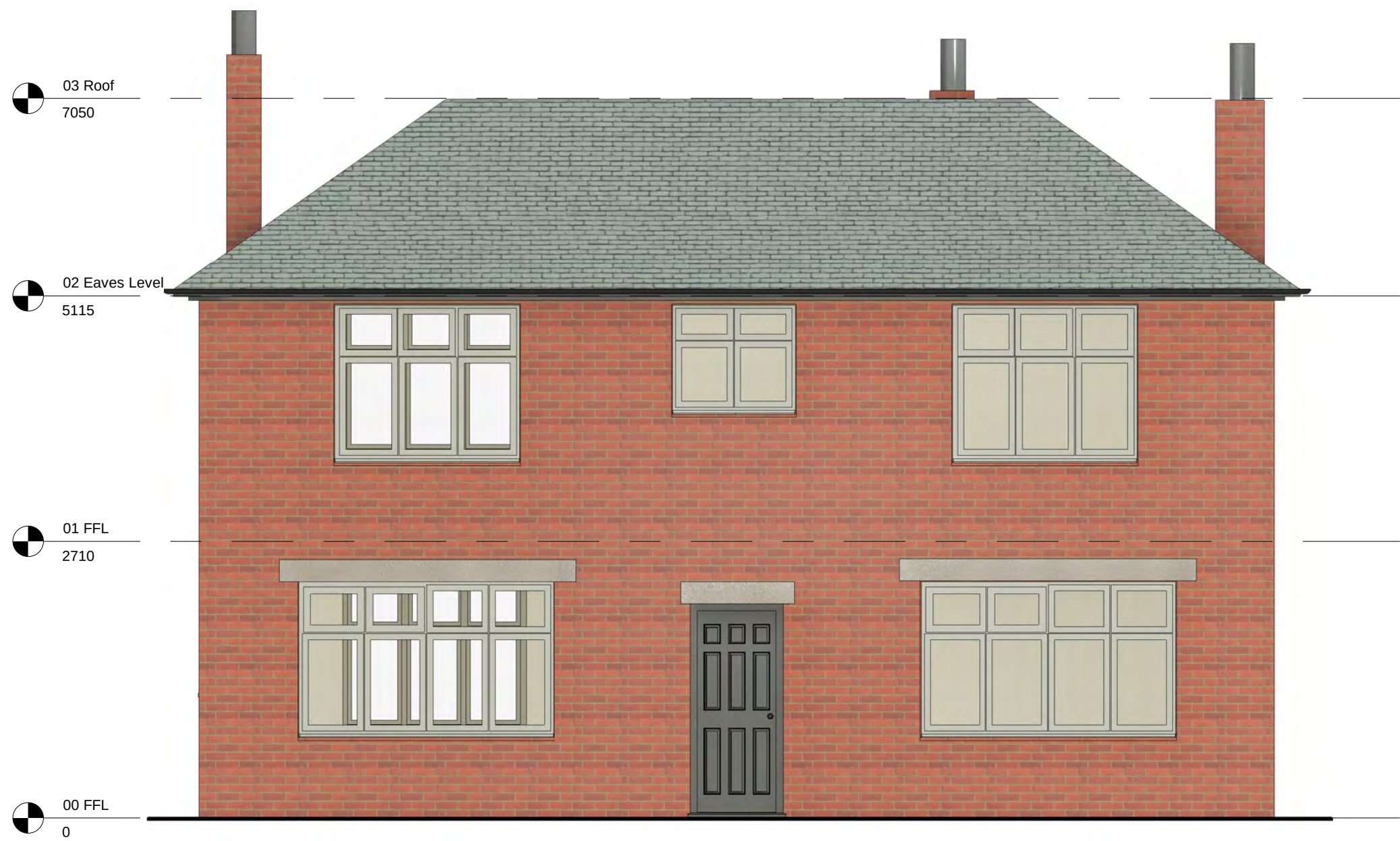
Existing Rear Elevation 1 : 50
