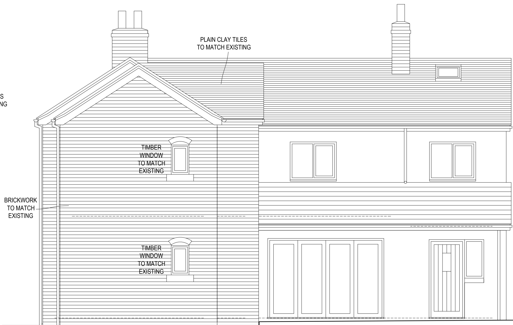
SIDE (NORTH EAST) ELEVATION / SITE SECTION - PROPOSED
