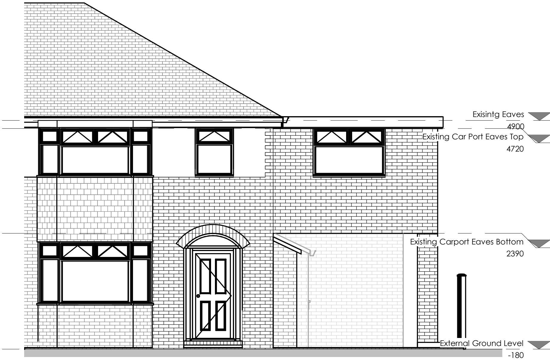
Existing West Elevation 1 : 50
