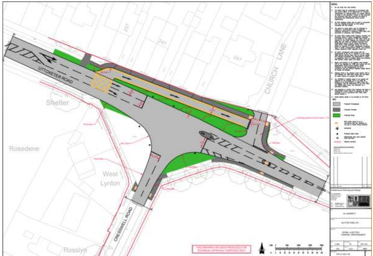
Fig 1.0. Proposed Uttoxeter Road Junction with Cresswell Lane
