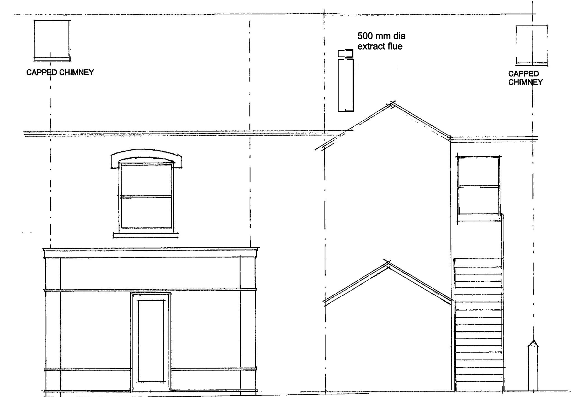
FRONT ELEVATION TO HIGH STREET
