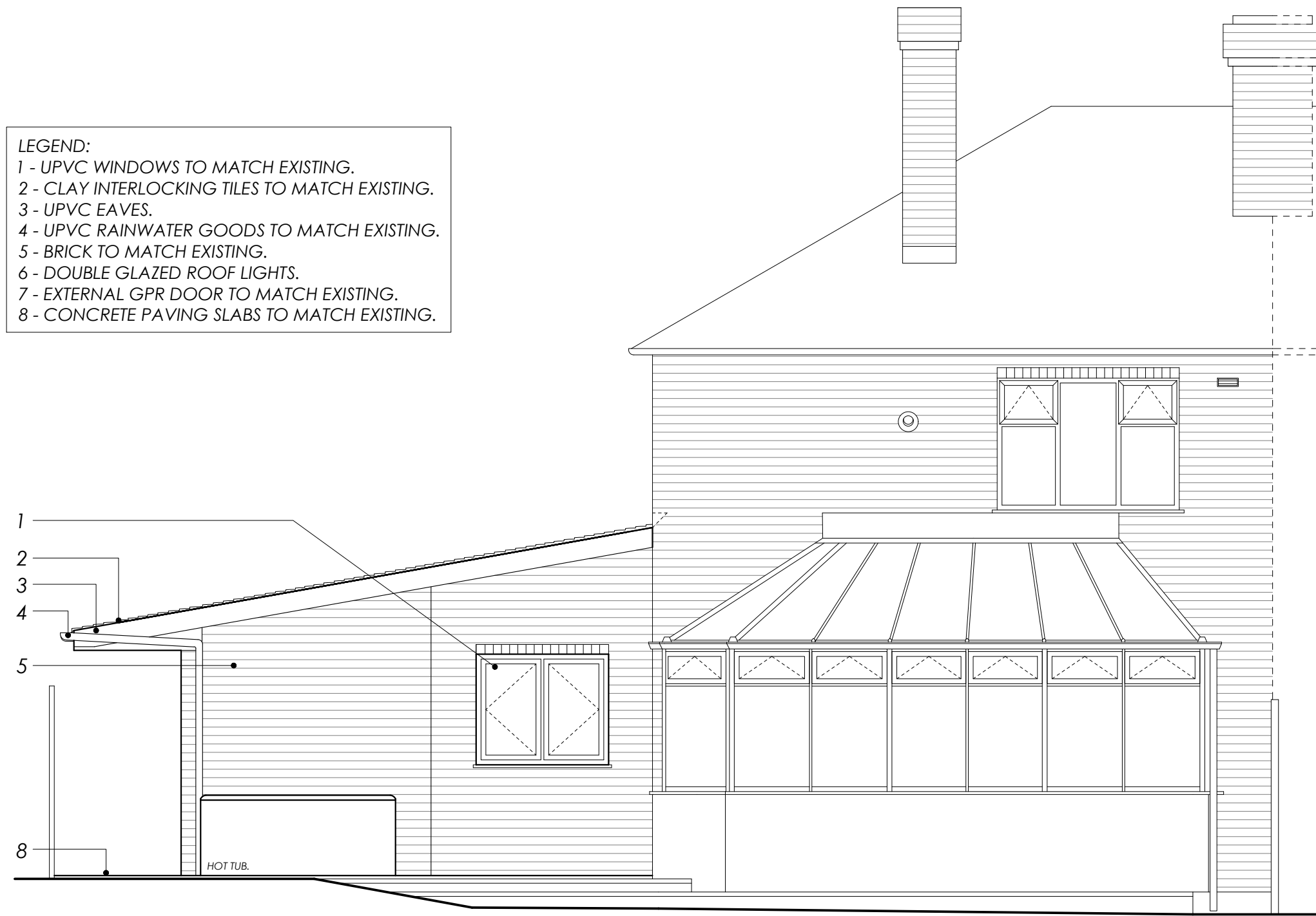
PROPOSED NORTH ELEVATION C 1:50 @ A1
