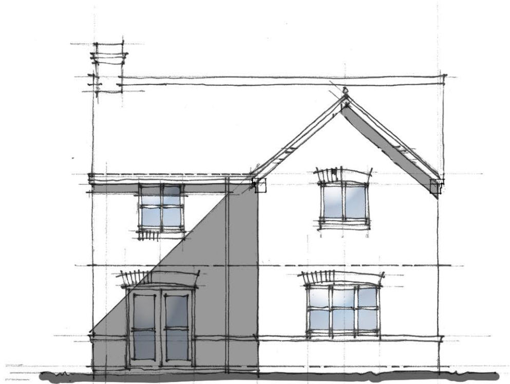
Proposed Rear Elevation [House Type E] [Scale 1:100]
