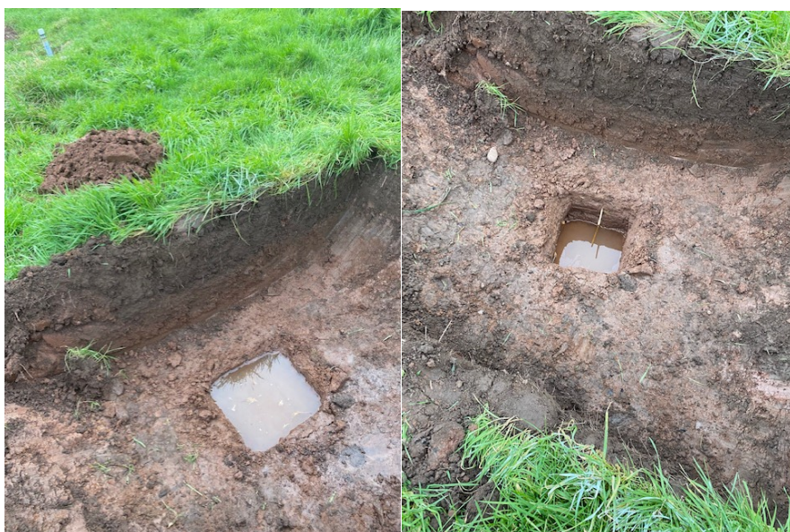
Trial Pit 2 – 500mm below surface - Before and During Test 50% Full level
