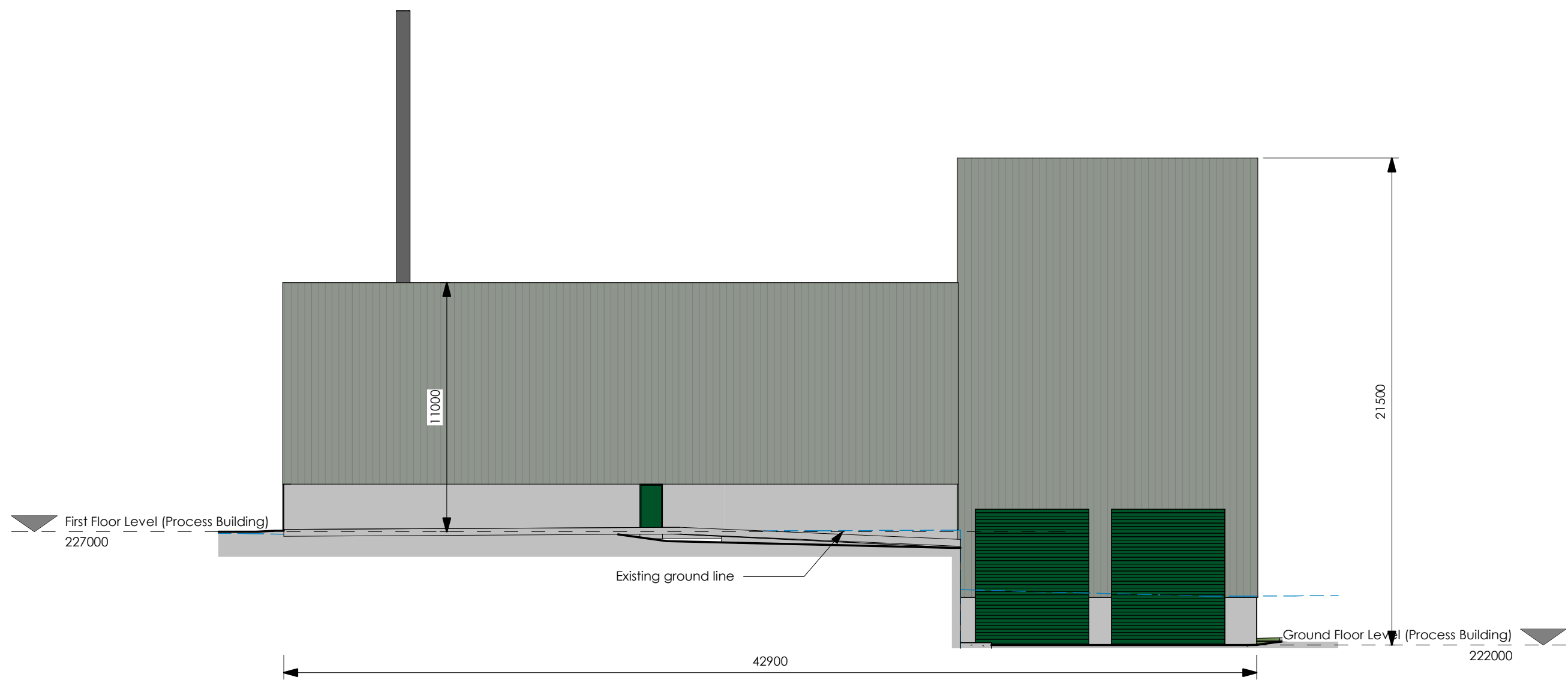
Proposed North West Elevation (Process Building)
