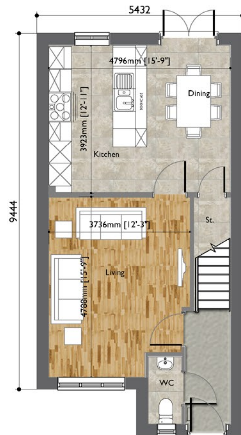
Ground Floor Plan Scale 1:100
