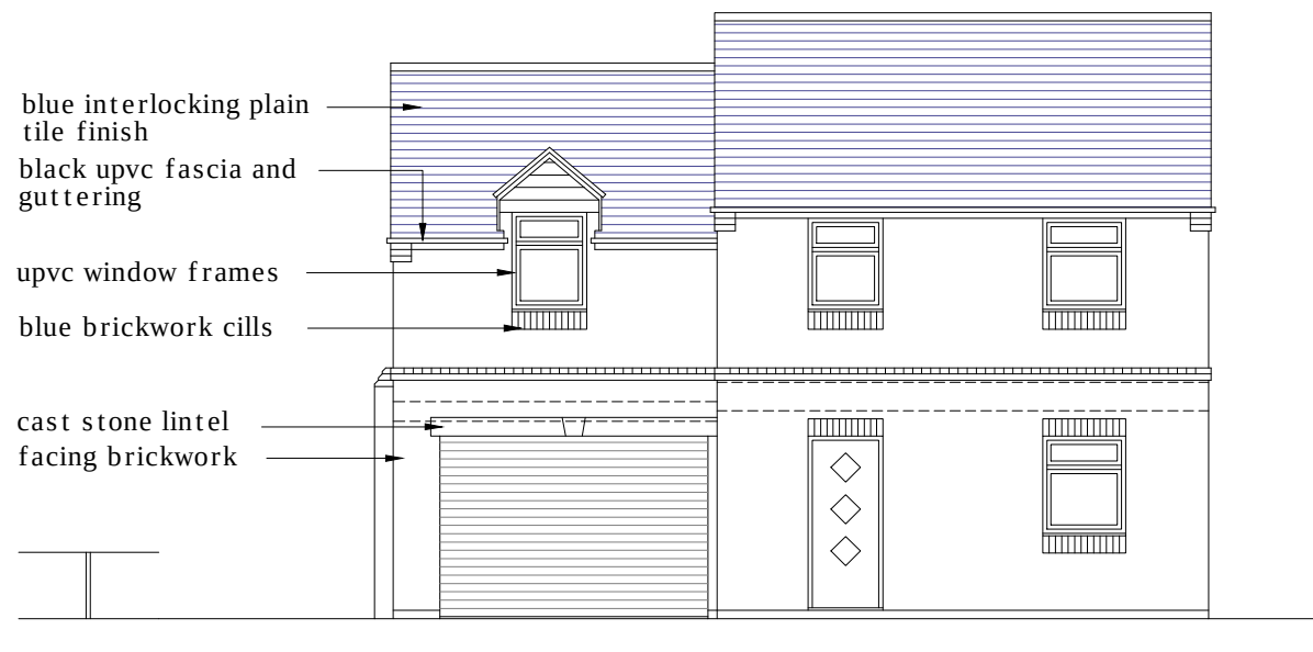
EXISTING NORTH EAST ELEVATION
