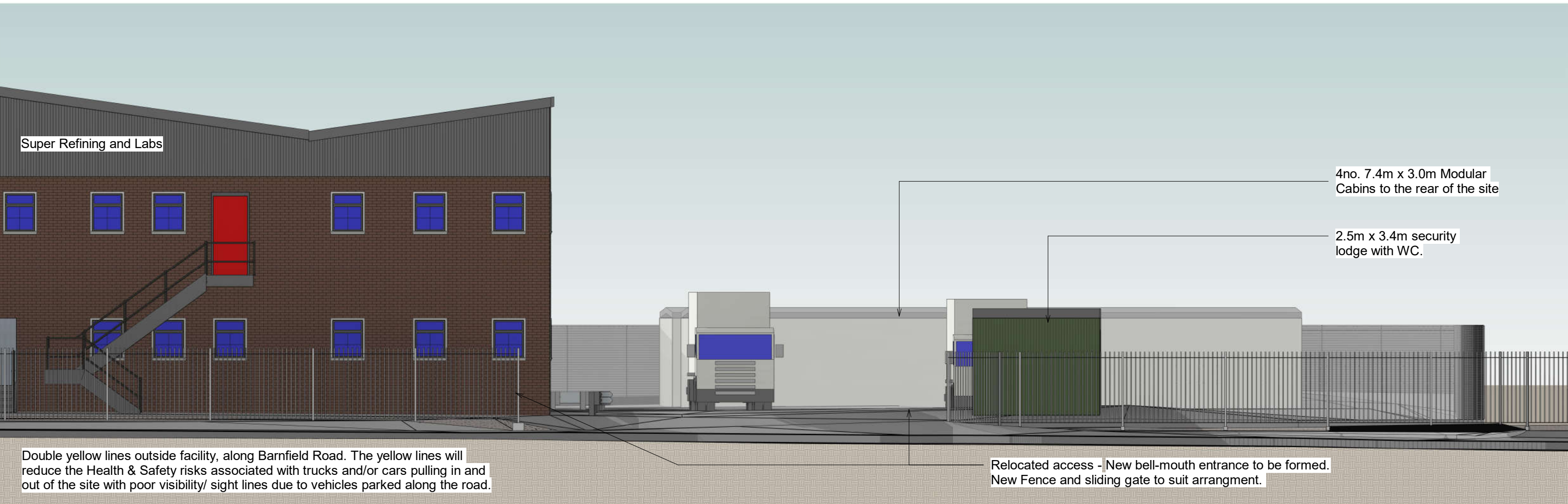
2 Elevation 2 - Barnfield Road - Exit 1 : 100
