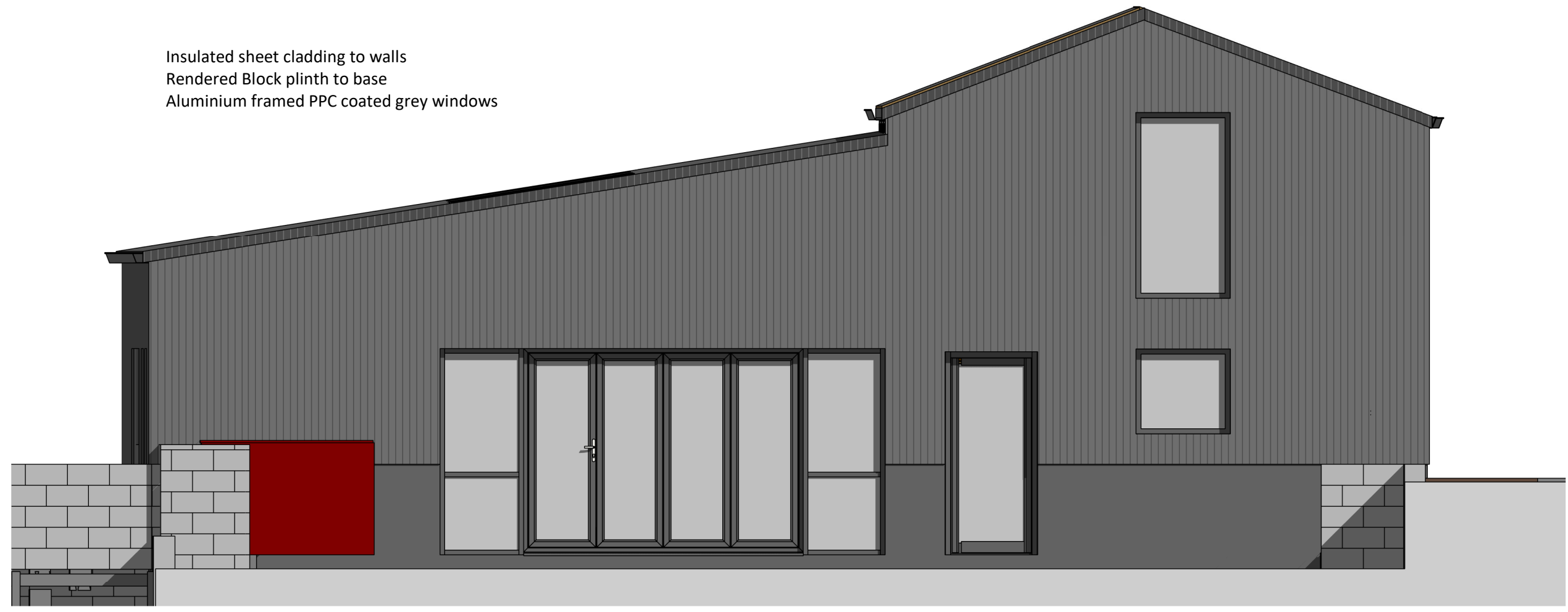
Proposed East Elevation
