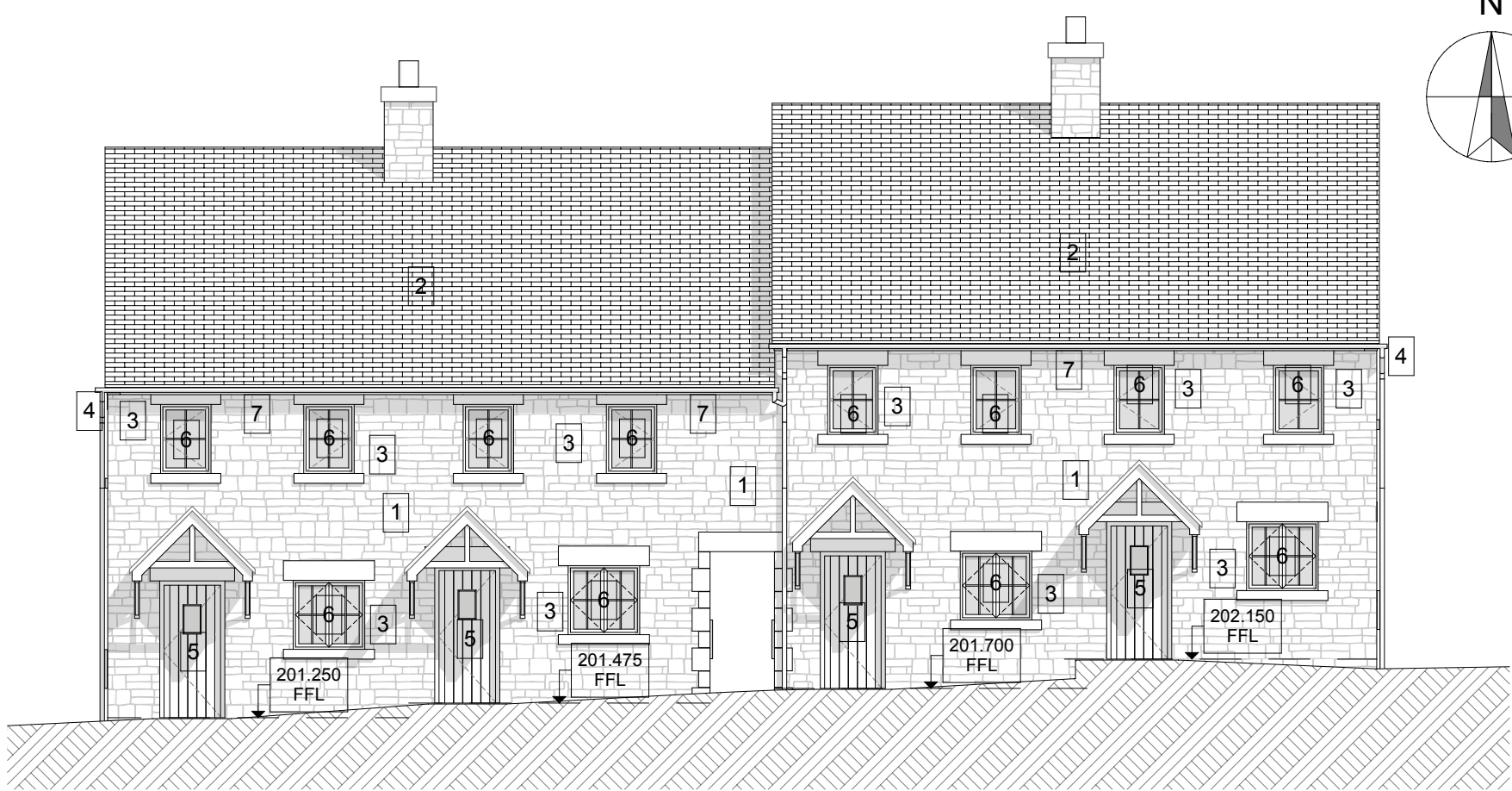
Proposed North East Elevation Plots 1 - 4
