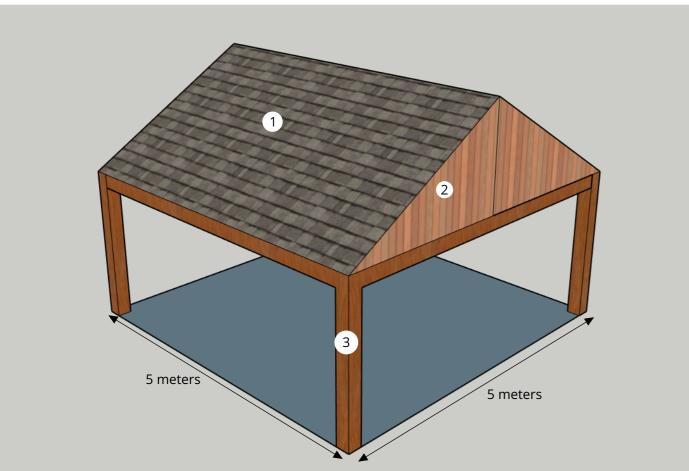
Oak carport with a felt tiled roof 5 meters x 5 meters square Total height of 3.7 meters Eaves height of 2.2 meters Roof Height 1.5 meters Zachary Hall 16 Friars Close Cheadle ST10 1AT 07720990480 zachal00@gmail.com
