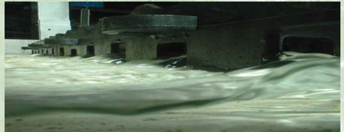
The SCS INTEGRA system has the unique benefit of full scale independent physical hydraulic modelling, providing the necessary data for developing validated porous paving designs on a scientific basis.
