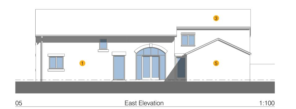
1 Stonework 2 Timber Cladding 3 Plain Tiles 4 Zinc standing seam 5 Brickwork
