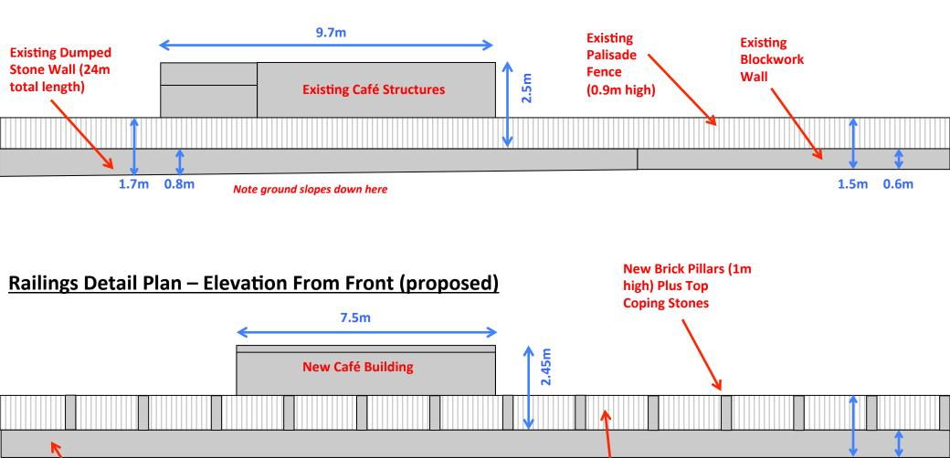
New Brick Wall (37m total length to replace blockwork in front of signalbox – see photos\_)
