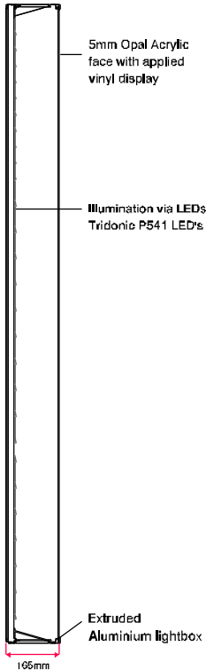
SECTION THROUGH scale 1:20
