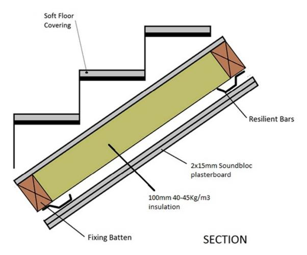
We would suggest the continuous use of the floating floor for the separating floor to be used in the place of the soft floor covering for "best practice" across the development. However were this is not practical, the minimum that should be used is the 6mm thick soft floor covering over the stair treads, as suggested in Approved Document E 2003. The 6mm soft floor covering should be bonded to the stair tread. Examples of a 6mm soft floor covering may include 6mm Hushmat.
