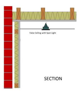
1. Downlighters and recessed lighting can potentially be used within the ceiling layers of the separating floor. However the chosen separating floor must be capable of allowing this.
