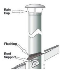
The roof support will be a black plate with black flexible rubber flashing seal set within the roof tiles. The visible pipe and rain cap are to be of black powder coated finish, this is commensurate to the existing external pipes on that side of the building. Thus maintaining the overall character of the building, and ensuring that the material of construction are of good quality.
