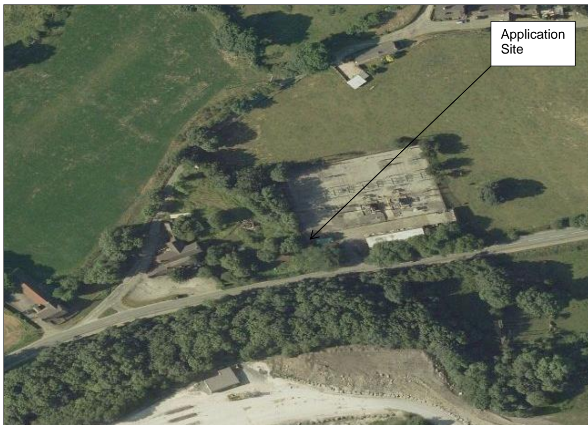
Figure 5: Caudon Grid Substation, bird's eye view looking north. The 33kV/11kV switching and transforming apparatus is sited in a secure compound in the open air, with the local transformer and control equipment in the buildings within the site. For safety reasons, the application site is at the southwest corner of the site adjoining the entrance, where it is distant from the switching and transforming apparatus. It is proposed to site the 15m tower in a location where the tower is screened by existing mature trees from both the road and the listed Yew Tree Inn to the west.
