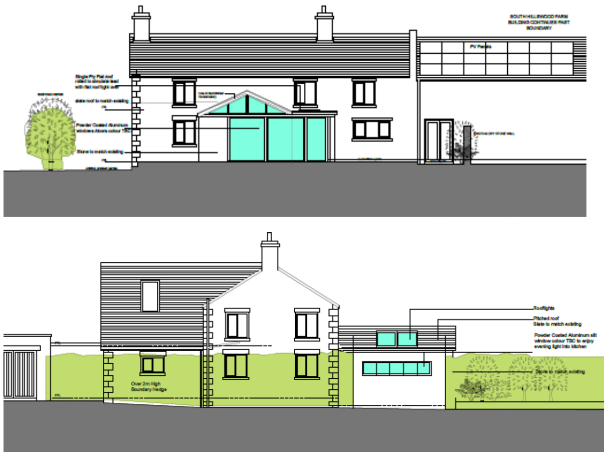
Fig.11 Revised Scheme – Utilises pitch roof, eaves and ridge heights of the existing conservatory to avoid the upper floor fenestration and with the reduced width allows a larger proportion of the existing elevation to be visible.
