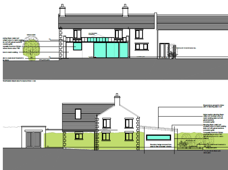
Fig.9 Pre application Scheme – Lean to roof back to Southern elevation roof had to articulate to avoid conflict with upper floor fenestration
