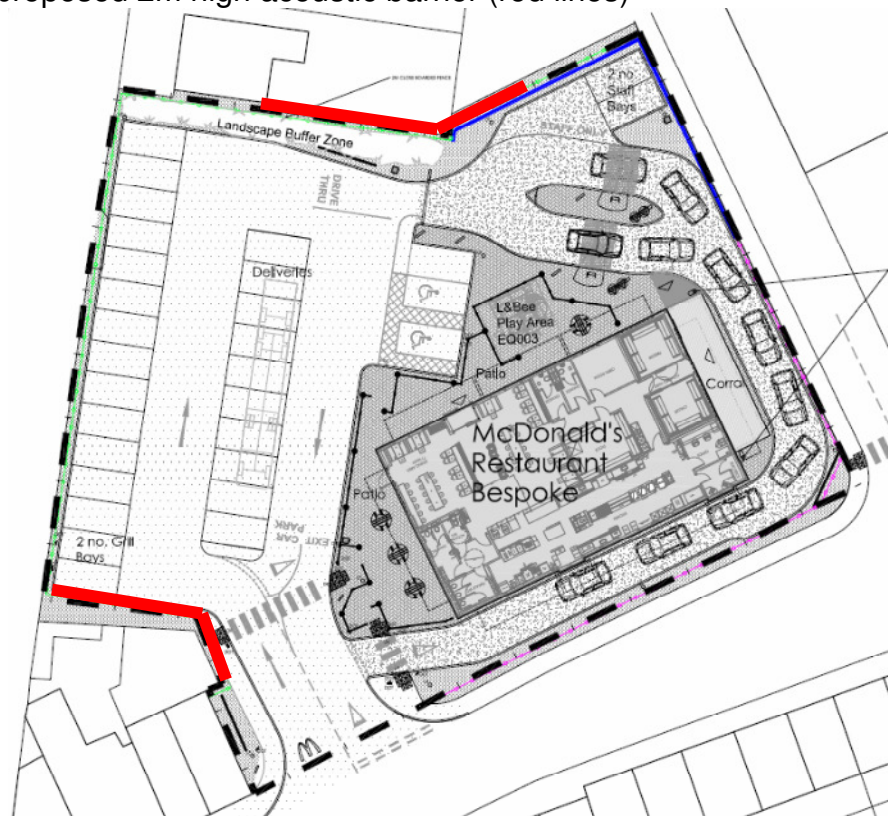
Figure 2. Proposed restaurant site layout, showing recommended extent of proposed 2m high acoustic barrier (red lines)
