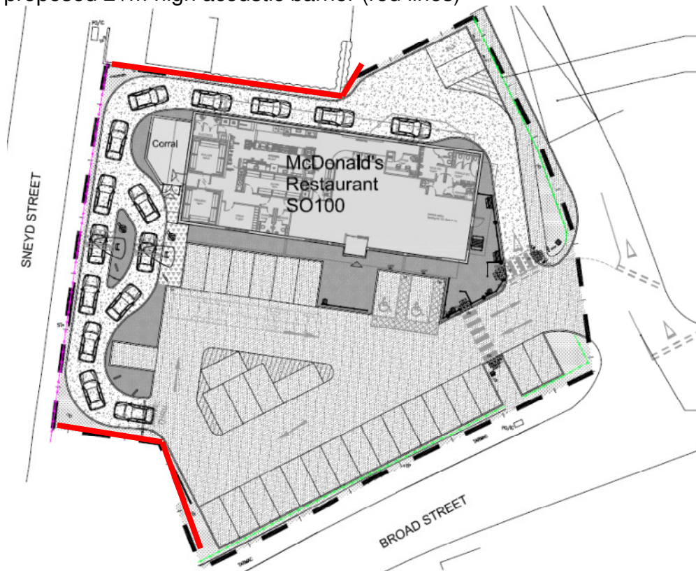
Figure 2. Proposed restaurant site layout, showing recommended extent of proposed 2+m high acoustic barrier (red lines)
